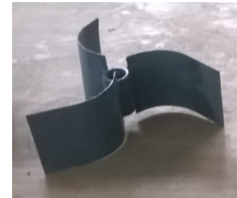
Model 1 Runner Formulated as Cross flow runner
