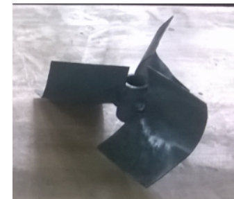
Model 3 Runner: Modification of Model 2 31
