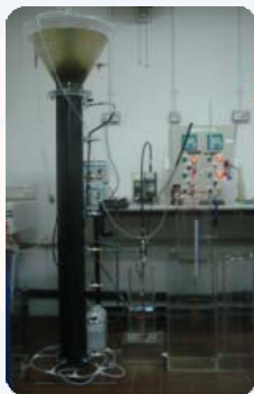
Upflow Anaerobic Sludge Blanket (UASB)
