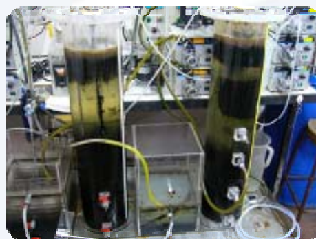
Sequencing Batch Anaerobic Reactor (AnSBR)
