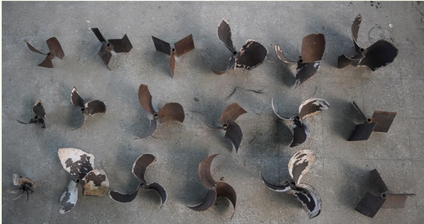
Figure : Various Runner Fabricated for Experimental Study
